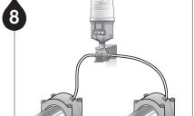
For typical bearing applications, install the divider block to the equipment using either copper or nylon tubes.
