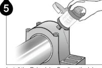
Install the Pulsarlube S unit on the lube point.
