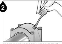
Ensure a clear passage using a manual grease gun. Note: Remove any hardened grease by purging the lube point with a manual grease gun. Note: The grease in the equipment and the grease contained in the unit should be the same or compatible
