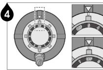
Turn the control knob to #5 to make sure the lubricator is dispensing properly. After checking, turn the control knob back to 'OFF' position.
