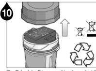
The Pulsarlube E is an eco-friendly product that can be disposed of separately. Turn the housing cap counterclockwise to disassemble the product for proper disposal.
