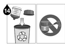
Warning Do not cut, puncture, or reuse lubricator.
